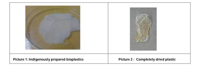
**Solubility test:** Solubility test was performed after bioplastic was completely dried. It was found to be insoluble in water. It is performed to check whether the prepared bioplastic dissolves in water or not. Since it was found to be insoluble in water, it indicates that it is suitable for use and it can be considered as a safe option to substitute the normal plastic. It can be improvised further to substitute the normal plastic.
