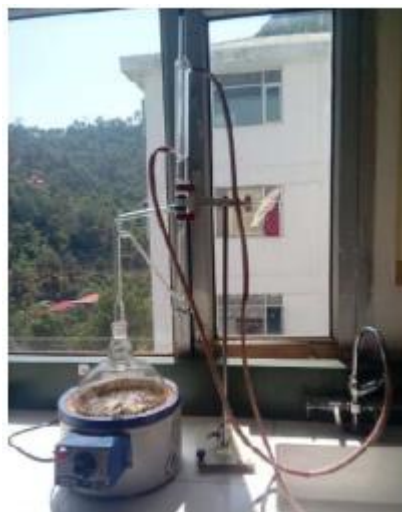
Figure 1: Extraction of oil through clevenger apparatus
