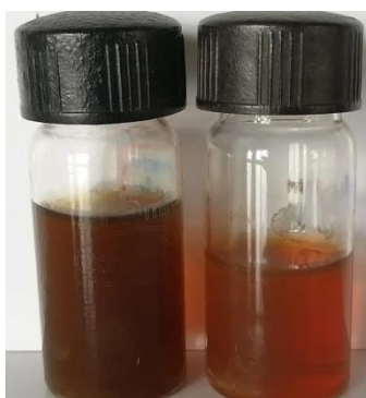
Figure2: Color change was indicate the presence of silver nanoparticles
