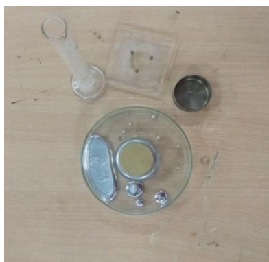
Fig.3 Shrinkage limit test apparatus& sample
