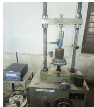
Fig.5 UCS apparatus during testing of soil specimen
