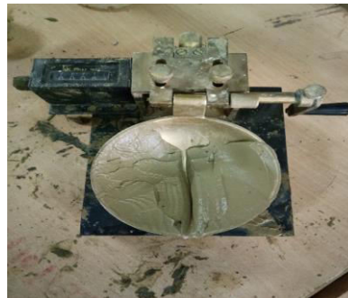
Fig. 2 Liquid limit apparatus during testing
