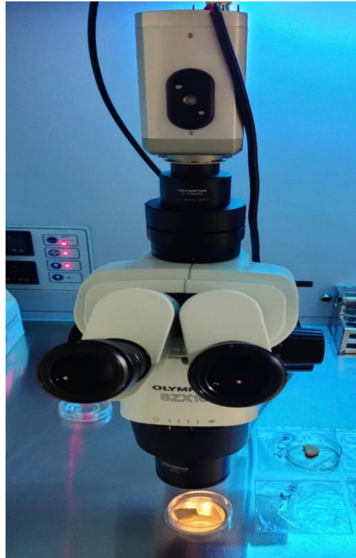
FIG8: Sectioned sample placed under stereomicroscope
